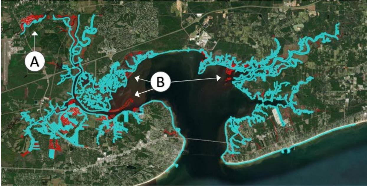
Figure 4: Choosing a feature length selection threshold for Inclusion of long features (units are feet): The selection of the 20 longest features (> 15,500) includes an unwanted, disconnected feature (A) and fails to include desired shorter features that contribute to the shoreline (B). Source: Esri, Maxar, GeoEye, Earthstar Geographics, CNES/Airbus DS, USDA, USGS, AeroGRID, IGN, and the GIS User Community.
