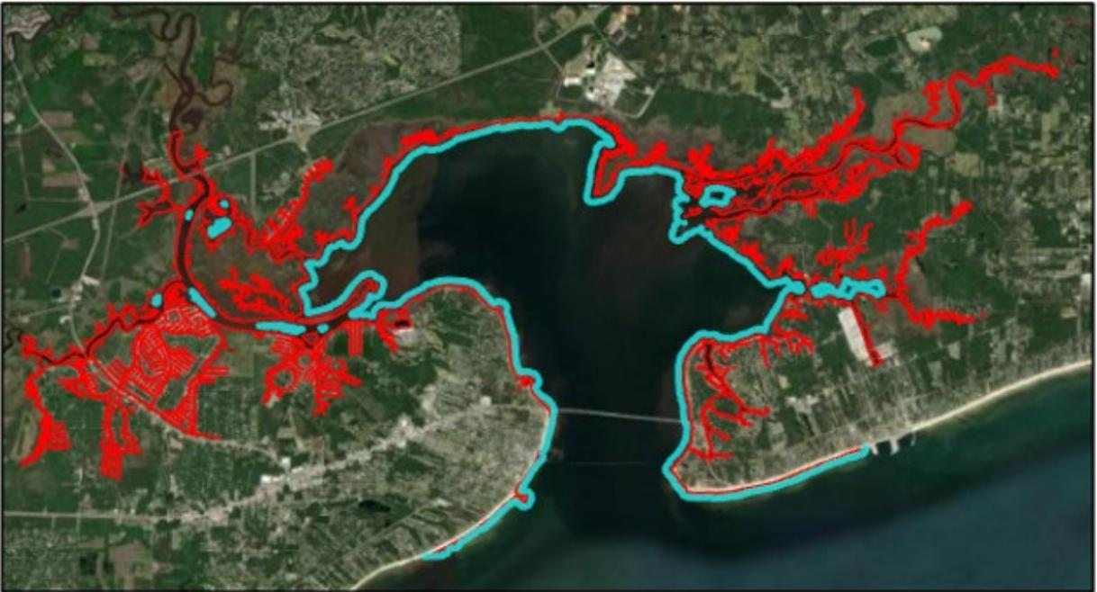
Figure 6: After converting the polygon to line, the line is split at the two points where the buffer intersects the shore (A, Top, is one example), then all lines representing the buffer over the water surface are selected and deleted (Bottom). Image Source: Esri, Maxar, GeoEye, Earthstar Geographics, CNES/Airbus DS, USDA, USGS, AeroGRID, IGN, and the GIS User Community.
